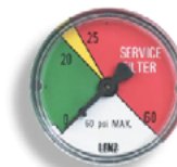
MC-20 RETURN LINE INDICATING GAUGE FOR 25 PSI FILTER APPLICATIONS 2" MULTICOLOR 0-20 PSI GREEN 21-24 PSI YELLOW 25-60 PSI RED (SERVICE FILTER)
